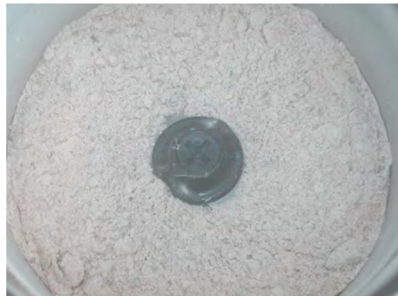
Fig. 4: Sample after fine-grinding in GM 300
