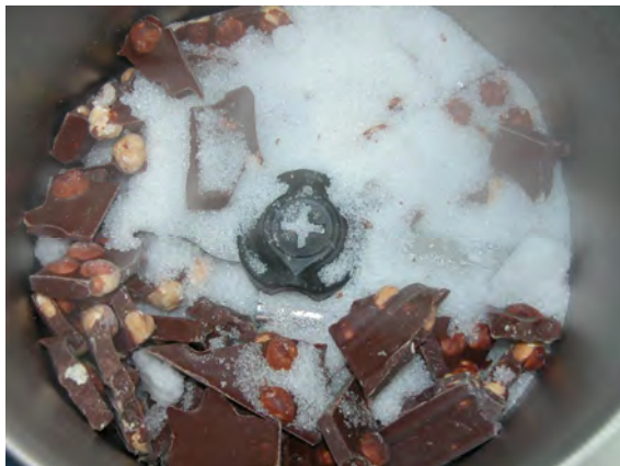
Fig. 3: Sample + dry ice in Cutting container GM 300
