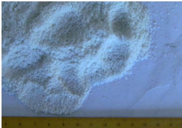
Fig. 3: Preform after fine grinding in ZM 200
