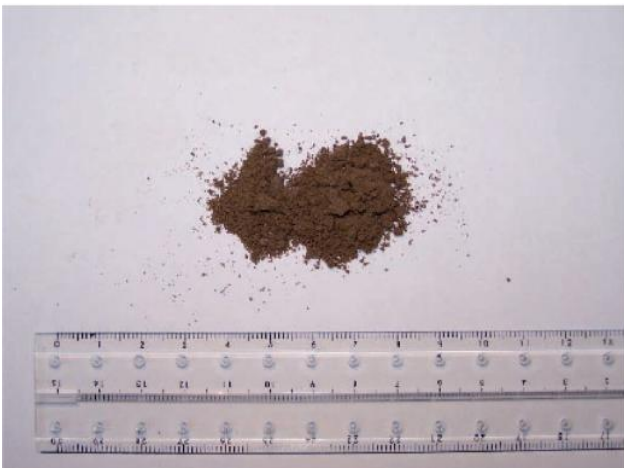
Picture 3: Sample after comminution in MM 400
