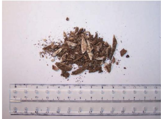
Picture 2: Sample after primary size reduction in BB 50
