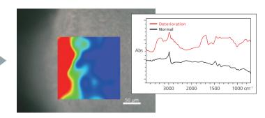
$\label{eq:maging} Imaging \mbox{ in the area} \\ \mbox{of the C} = O \mbox{ peak indicating oxidation degradation} \\$
