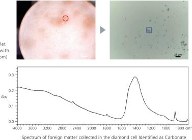
Observation image of the foreign matter on the diamond cell by 15× Cassegrain objective mirror.
