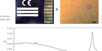
Observation image of the foreign matter on the terminal by 15× Cassegrain objective mirror.
