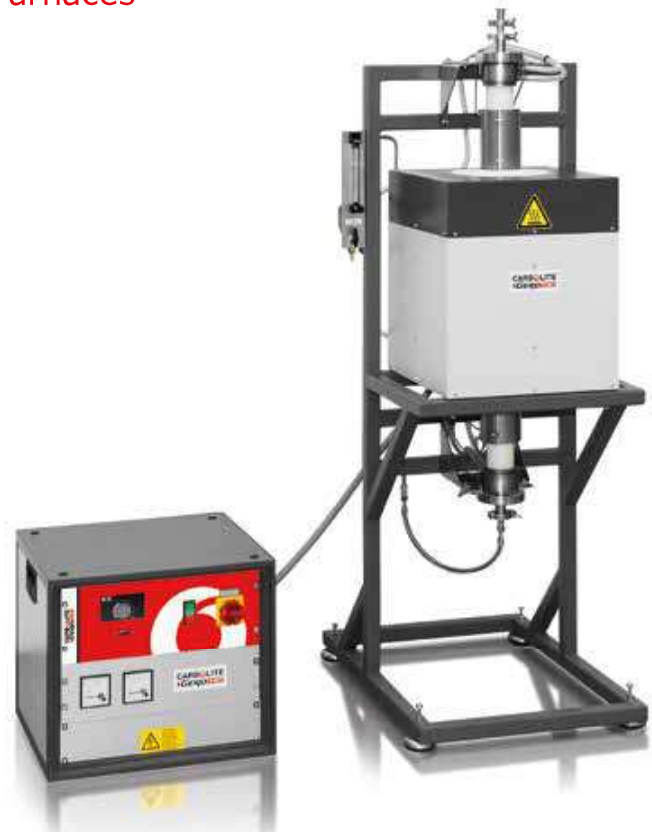
HTRV 18/70/250 with optional CC-T1 controller, optional 'L' stand, optional voltage/current display and optional high vacuum/inert gas package (high vacuum possible up to 1450 °C). Rotary vane and turbomolecular pumps available as options.
