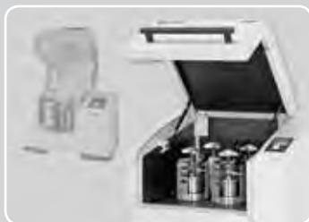
Fine size reduction with impact and friction can also be carried out with RETSCH Planetary Ball Mills. They are used for **larger sample volumes** and **colloidal grinding** and achieve grind sizes down to the submicron range.
