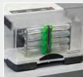
Grinding jars of polystyrene are also available for the mixing of solid sample materials.
