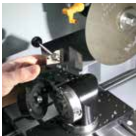
Swivel unit with fast lock vice 50
