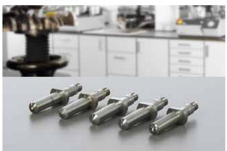
The various indenters are to be selected according to the respective test method (Brinell, Vickers, Rockwell and Knoop). The selection of QPREP indenters, test diamonds and carbide balls, which are certified according to DAkkS and/or ASTM, QATM, provides a broad test equipment portfolio for hardness testing.
