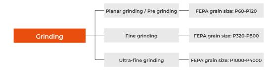
Typically, silicon carbide (SiC), aluminum dioxide (Al2O3), silicon dioxide (SiO2), zirconium dioxide (ZrO2), diamond or cubic boron nitride (CBN) are used as abrasives. Particular attention must be paid here to low-deformation material removal and at the same time to keeping the number of preparation steps as low as possible. A wide range of QPREP grinding media is available for this purpose.
