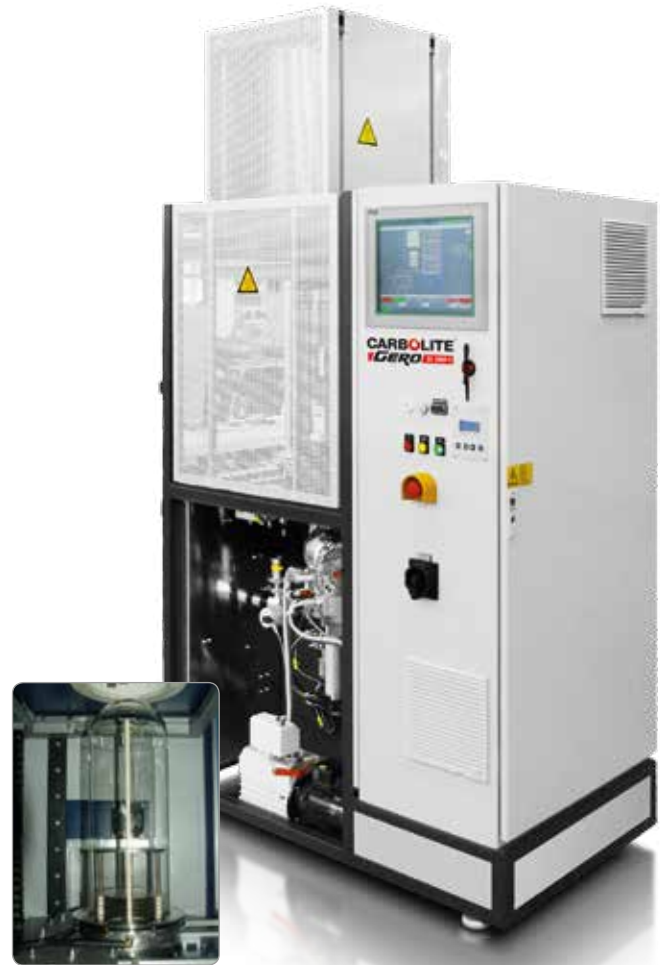
Tube furnace in the upper position. The quartz recipient stays at the bottom and is still connected to the vacuum pumping unit.
