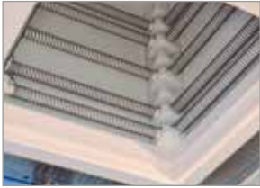
Picture inside the hood of the HB equipped with CrFeAl heating elements for a maximum temperature of 1300°C.
