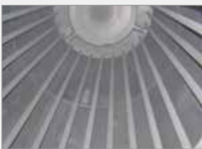
Picture of the mantle heater made from graphite. It consists of several graphite rods, which are arranged symmetrically to ensure a uniform temperature distribution.
