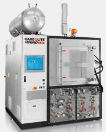
HTK 25 W/22: High temperature chamber furnace with a usable volume of 25 l up to 2200°C with automated operation via a touch panel interface.
