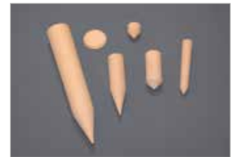
Ceramic crucibles for Bridgman growth
