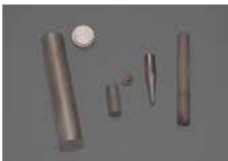
Graphite crucibles for Bridgman growth
