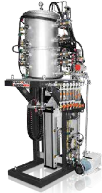
KZA-V 25-500/20: Bridgman crystal growth furnace with a heated length of 500 mm up to 2000°C. 4 zone graphite heaters for vacuum and inert gas operation with fully automatic control and data logging.
