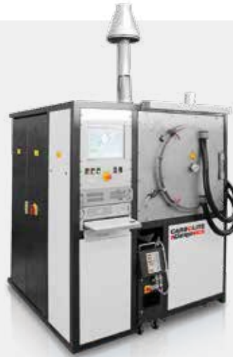
EBO 120/1.5: Debinding furnace with a usable volume of 120 l up to 150°C at most. The required working temperature is 120°C. Nitric acid is evaporated, mixed with Nitrogen and purged into the furnace for catalytic debinding.
