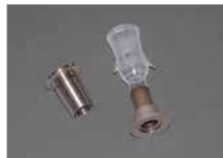
Glass-metal transition pieces for vacuum connection
