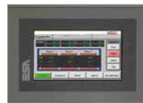
Touch panel interface for furnace control and process visualization.
