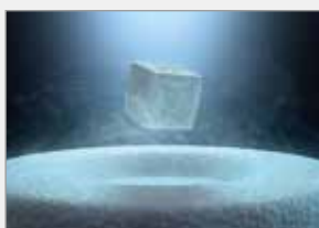
Levitating superconductor due to the compensation of the magnetic field inside of a superconductor.
