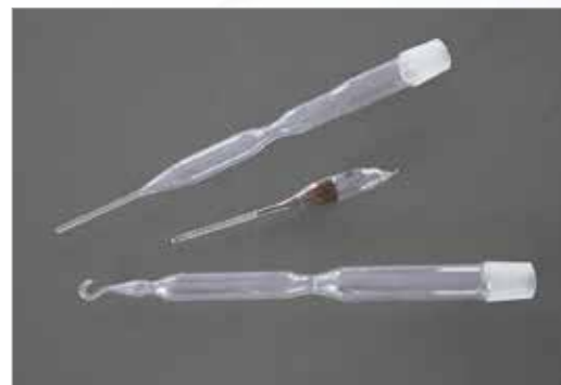
The Bridgman ampule with a tip and rod is shown above. The ampule melted and closed at one side is shown in the middle. The tip serves to generate the crystal growing seed when passed through a thermal gradient. The ampule with a clamp is shown below.
