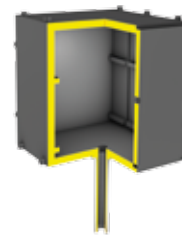
Graphite retort with a gas outlet tube
