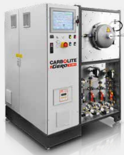
GLO 40/11: Furnace with a usable volume of 40 l up to 1100°C under atmospheric pressure. The GLO is used for thermal debinding.
