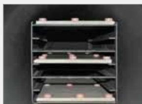
Zoom inside: Charging rack inside the retort
