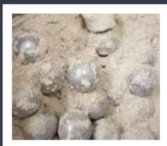
140 g dried mushrooms were ground to 100 µm in 90 min at 60 min<sup>-1</sup>, in a 10 l drum with 10 kg of 20 mm stainless steel grinding balls.
